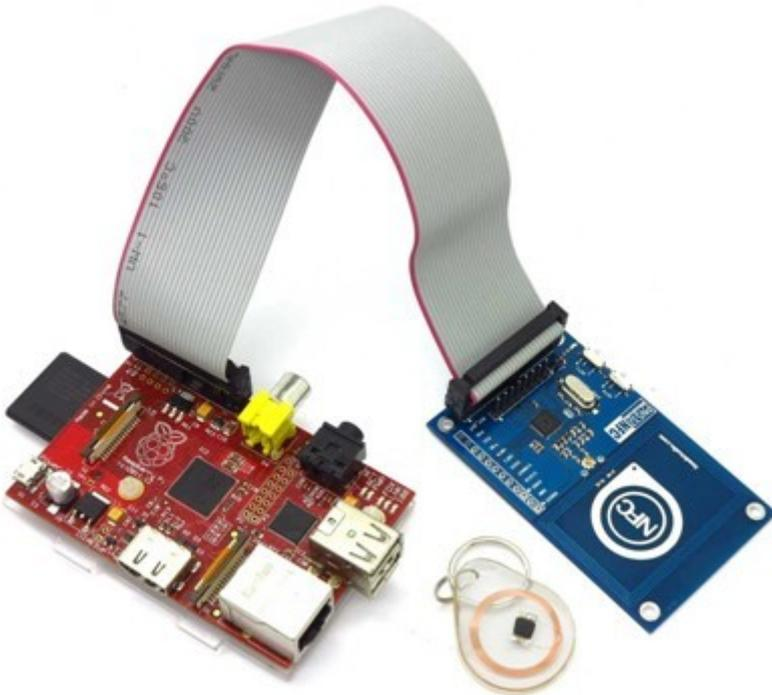
According to the connection in the picture above, Itead PN532 Module is connected via the SPI bus with raspberry pi, therefore, operating mode of PN532 Module should be set to SPI mode, as shown below:
