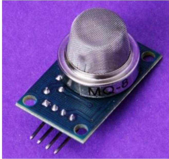
MQ-8 Hydrogen Gas Sensor Circuit Built with an Arduino
