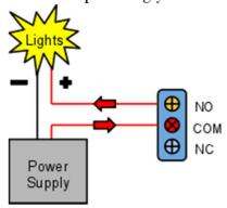
Example of connecting power and lights to a relays COM and NO connectors.
