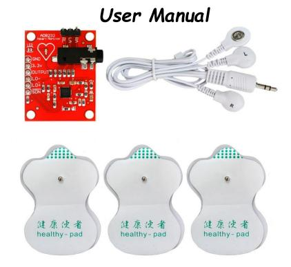
An ECG Sensor with disposable electrodes attaches directly to the chest to detect every heartbeat. The electrodes of ECG sensor will convert heartbeat to electric signal. ECG Sensor is very light weight, slim and accurate to measure continuous heartbeat and give rate data of heart beat. This device is used by trained doctors and medical assistances.
