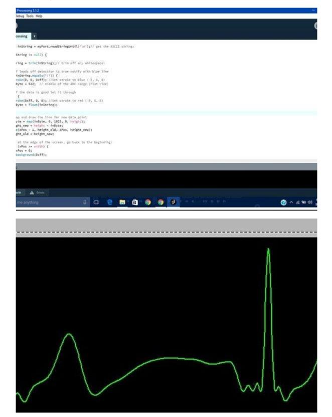
For graphical representation download and open .pde file in Processing. Select the baud rate same as Arduino.
