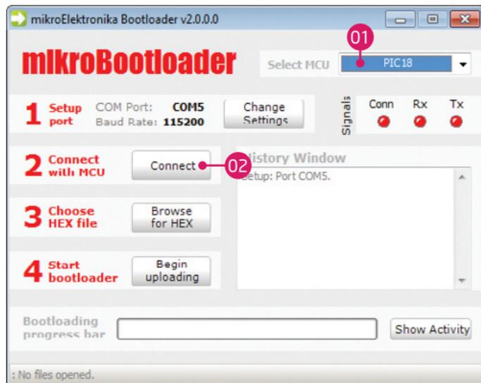
Figure 1-4: Connecting mikromedia with mikroBootloader
