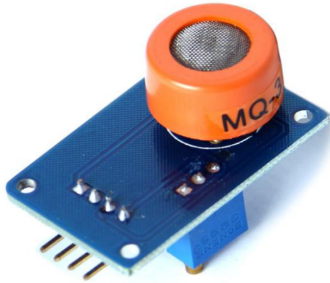
MQ-3 Alcohol Sensor Circuit Built with an Arduino:
