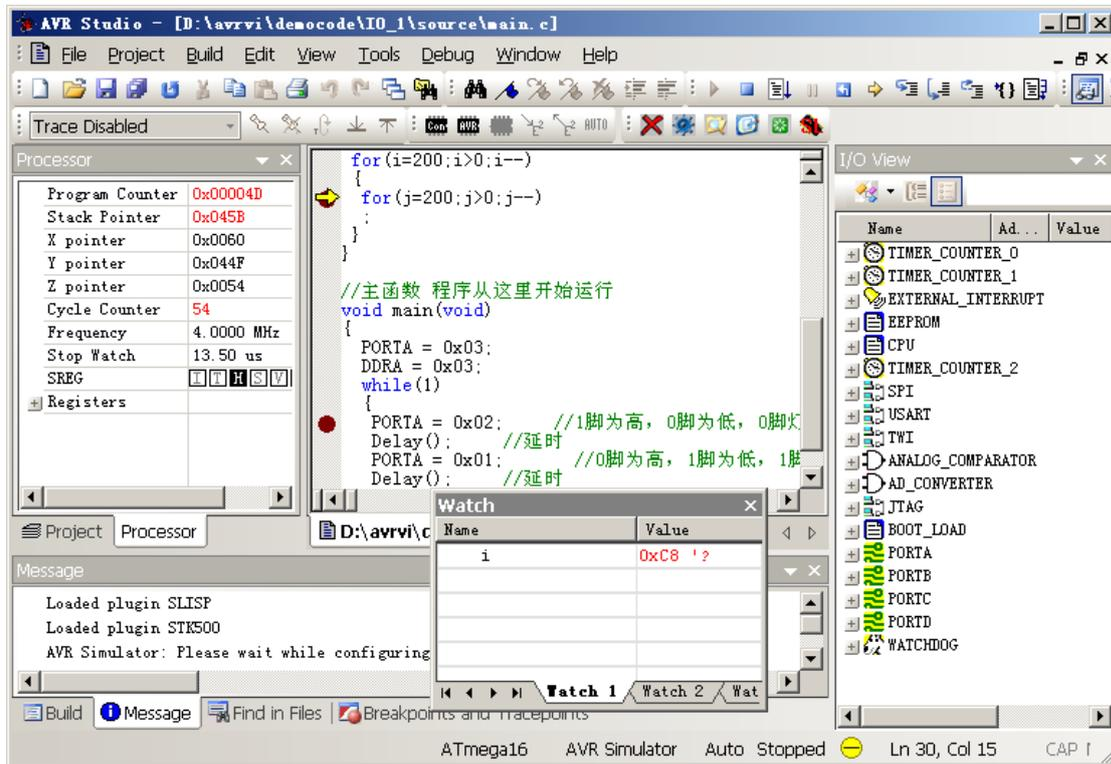
Here are code view, information view and processor etc. You can see the chip work station such as IO port, Timer, AD, USART etc. You can through the menu button to do single step debugging, set breakpoints, observe variables, see registers, check procedure of spatial data, etc.
