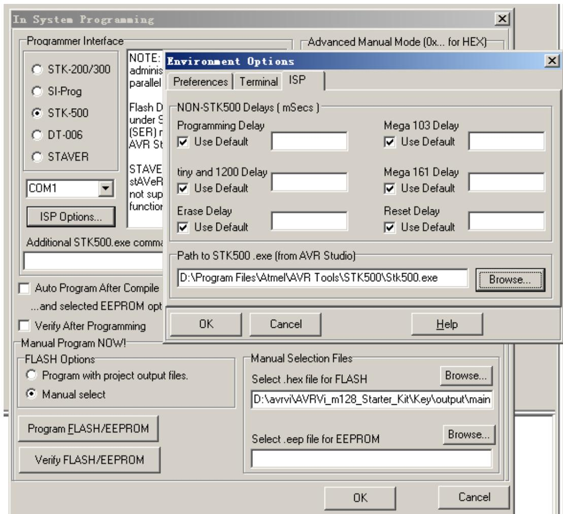
After the parameters set, you can program HEX and EEP file, and read or and program fuses and lock-bits. (Note: please do not change fuse setting until you know well about them, wrong fuse settings should lock the AVR chip.)
