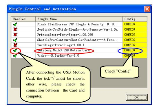
Check the "Config" to entry the "USB Motion Card"
