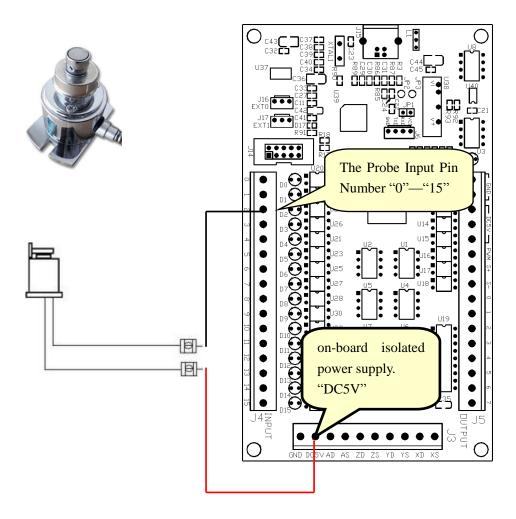
Setup Probe input signal, as shown below: (Config => Ports and Pins)
