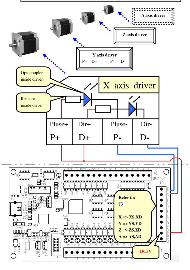
5.1.2 Using External power supply to drive.
