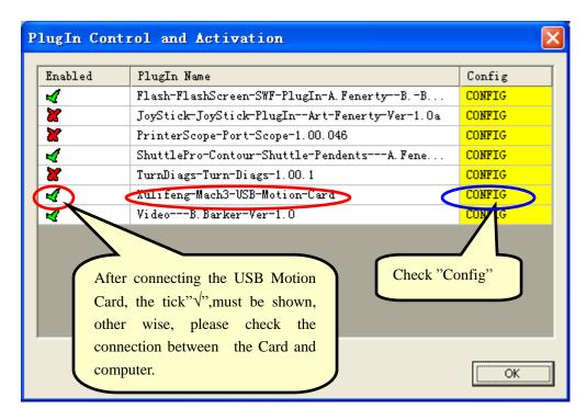
6.4 After check the "Config", USB Motion Card setting will be shown. You can select one of the functions which is able to controlled by the external knob. Please select "External 0" in your particular setting. Then, click "OK" to exit.
