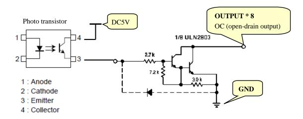
8 general-outputs, wiring of the 0, 1, 2, 3, 4, 5, 6, 7 on J5.
