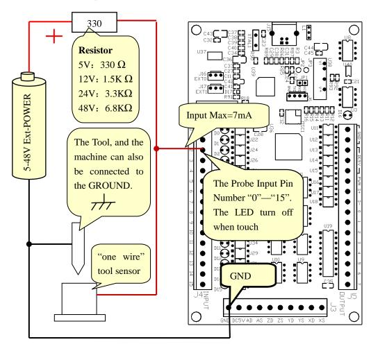
Setup Probe input signal, as shown below: (Config => Ports and Pins)
