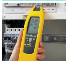
Location of fuses/breakers and assignment to circuits
