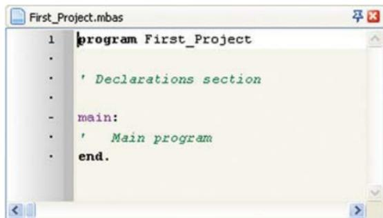
After creating the project, a new blank window to write a program in will appear. See Figure on the left. If you use *New Project Wizard* when creating a new project, a blank source file, named after the project with the *.mbas* extension, will automatically be created. The *mikroBasic PRO for AVR* does not require you to have a source file named the same as the project, it's just a matter of convenience.
