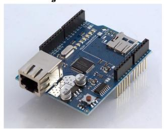
To use the shield, mount it on top of an Arduino board (e.g. the Uno). To upload sketches to the board, connect it to your computer with a USB cable as you normally would. Once the sketch has been uploaded, you can disconnect the board from your computer and power it with an external power supply.
