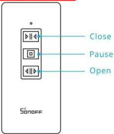
1- Power off the Curtain Motor, long press the pairing button and then power on the Curtain Motor to wait for about 5s until the LED indicator turns green and keeps on, then release. Now Curtain Motor has entered the Curtain Remote pairing state.
