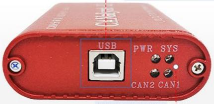
LED light set, indicating the running status of the equipment in the whole process
