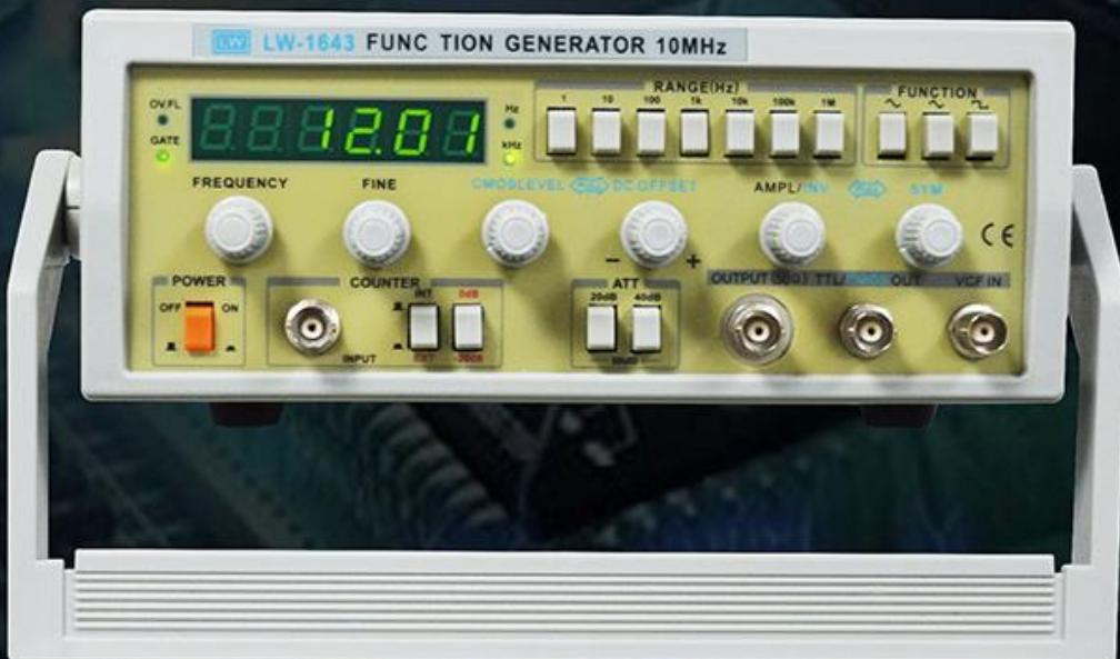
**TTL Pulse, low level higher than 0.4V, high level not less than 3.5V
