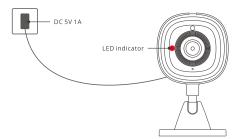
After powering on, the device is reset by default during the first use. The camera entered the pairing mode successfully when you hear the voice prompt "please use mobile phone for Wi-Fi configuration" and see the LED indicator turns to solid red.
