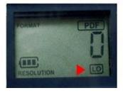
LO Resolution can raise scanning speed for scanning data files
