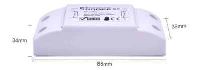
Modle : Sonoff RF Product Type : Smart WiFi Switch WiFi Standard : IEEE 802.11 b/g/n Support RF : 433MHz Voltage Range : 90-250V AC Max. Current : 10A Max Power : 2000W(Resistive load) Color : White Material : ABS V0 Product Size : 34\*88\*39(mm)
