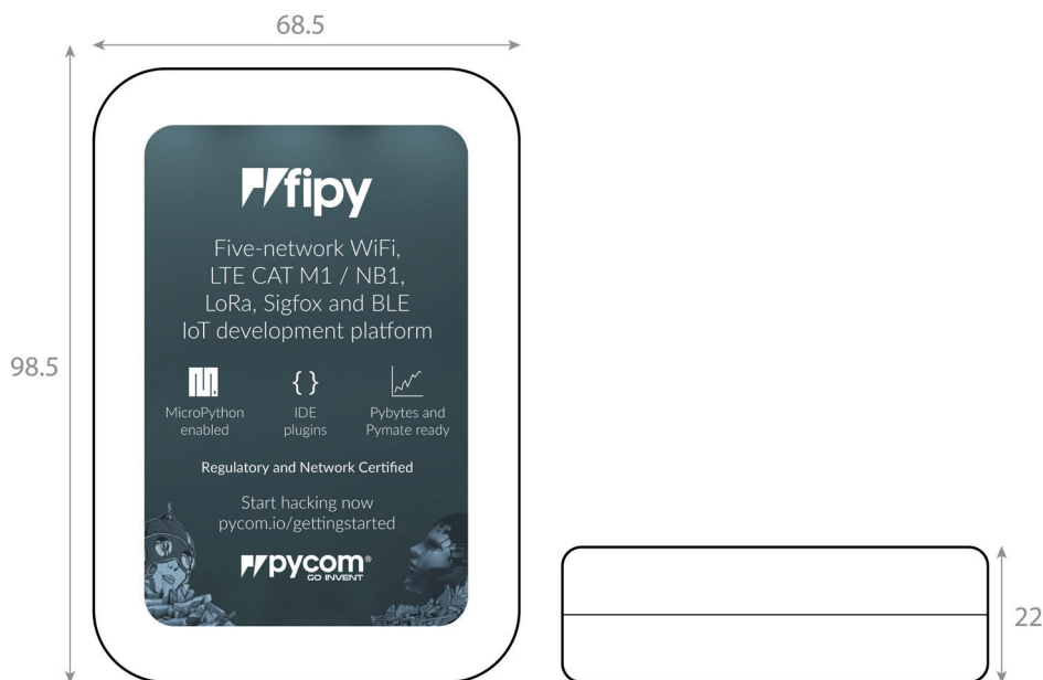
Figure 7 – Mechanical drawing of packaging – Units: mm
