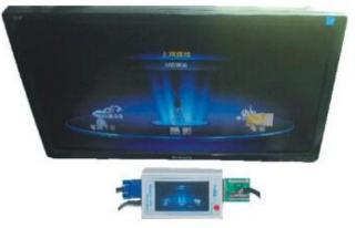
**Step 5**: After connection, if the mainboard of TV is normal, the display or external display on converter will display the image of mainboard of TV.
