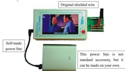
To facilitate the mainboard testing on site, a portable power source is able to be used to supply power to the converter. It is actually measured that Mi 10400 power (portable power from other brand is able to be selected) is able to supply power to this converter for 15 hours, fully conforming to testing requirements
