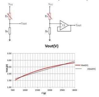
**Pressure Threshold Switch:** This is a typical application circuit that controls on and off by setting a specific pressure. It consists of a Wheatstone bridge and a voltage comparator. When the pressure increases so that the sensor resistance is less than R1, the voltage comparator U1+ is higher than U1- and outputs a high level. The high level of the output can be added to the device attached later.
