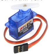
The FS90R is a micro-sized servo specifically for continuous rotation. It can be controlled using a direct connection to a single microcontroller I/O line without any additional electronics, which makes it a great miniature actuator for beginner robotics projects.
