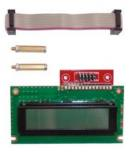
16  $\times$  2 character LCD module with mounting holes, pillars and 10-way ribbon cable for connection to MICRO-X board. MICRO-X kit comes with tutorials and sample code to program the LCD in assembler and C code. This module is green. LCD screen: 61  $\times$  16mm, PCB size: 83  $\times$  45mm.
