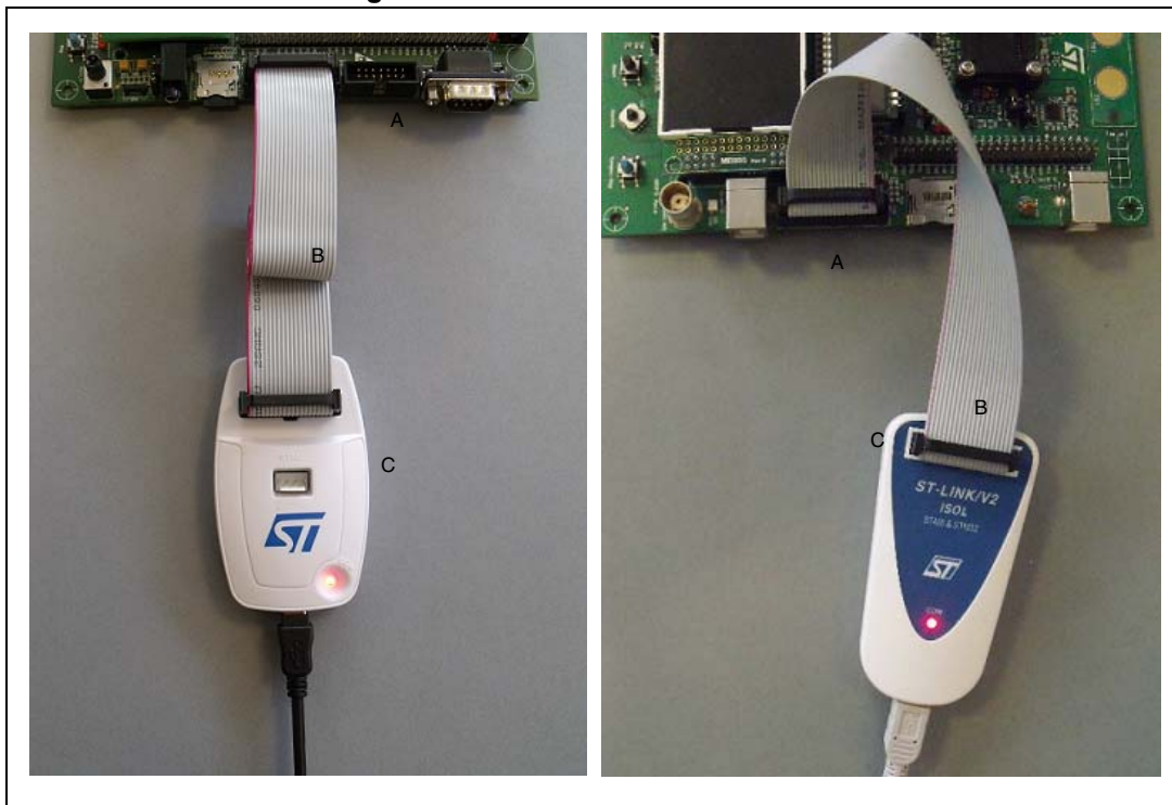
Figure 9. JTAG and SWD connection
