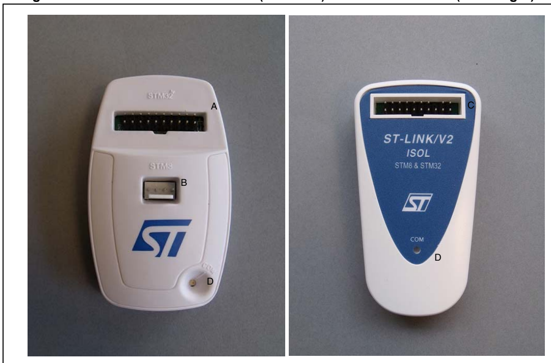
Figure 4. Connectors of the ST-LINK/V2 (on the left) and ST-LINK/V2-ISOL (on the right)
