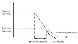
With regard to stop mode after stop frequency is reached, you can choose DC injection brake and other options. If you do not choose DC injection braking, it will stop in coasting stop mode.
