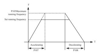
The Default Acc/Dec time is the primary Acc time/ Dec. time. Other Acc time or Dec time can be selected via external terminal.
