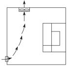
Correct installation position of the fan
