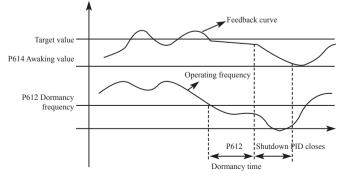
Example: PID action set point is 60% (0 – 100% is corresponding to 0 – 10V), and the wake-up value is 80%, which is actually corresponding to 0 – 10V, then the actual wake-up value is  $60\% \times 80\% = 48\%$  (corresponding to 0 – 10V).
