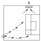
Incorrect installation position of the fan
