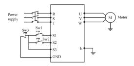
Use S1, S2, or S3 as input terminal for external signal Parameter: P317=6 S1 is in forward P318=7 S2 is in reverse P319=9 S3 is in stop mode P102=1 external terminal input
