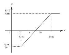
Introduction: P300=2 FIV minimum voltage input: 2V (inverter regards signals below 2V as invalid signals);
