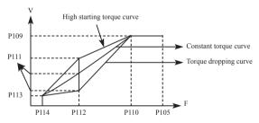
P109: V/F maximum voltage, V/F maximum voltage can be set according to the motor connected. Generally, it will be set at the rated voltage of motor. When motor is very near to inverter, usually within 30m, it should be set at a higher value.
