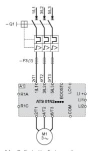
A1: Soft start/soft stop unit(1) For type 2 coordinationQ1: Motor circuit-breakerF3: 3 fast-acting fuses
