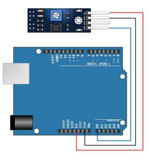
You actually don't even have to write any code to start using the Arduino TCRT5000 sensor, all you need to do is launch the AnalogReadSerial example and Upload it to your Arduino.
