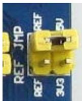
Figure 18: Setting AD reference voltage
