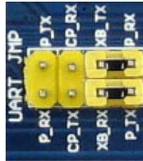
Figure 14: Setting jumpers on ARPI600
