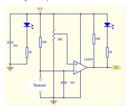
This light sensor uses a Cadmium Sulphide Photoresistor as a sensor. It then amplifies the signal and outputs:
